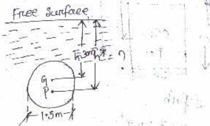
Given data :- Dia of plate  $d = 1.5 \text{ m}$
