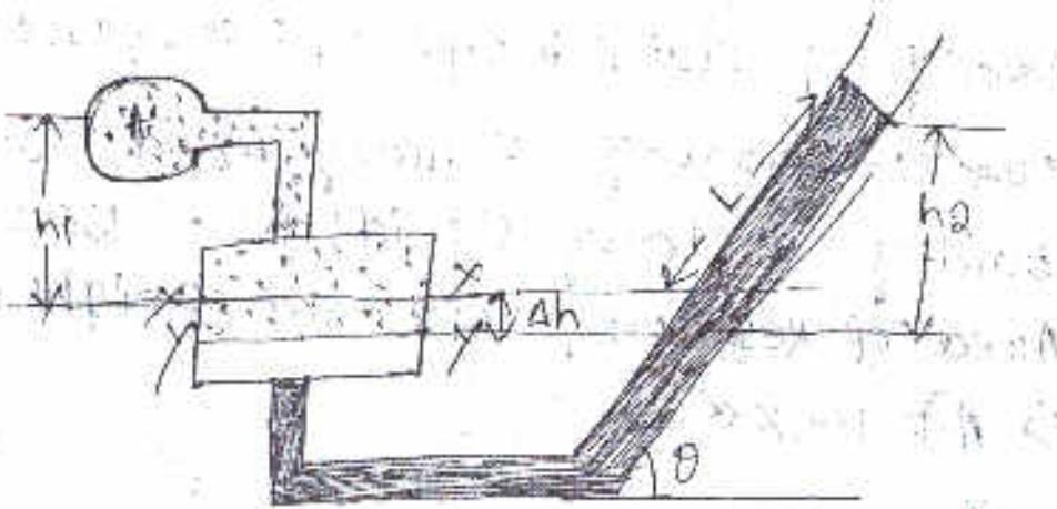
→ It is a modified form of a U-tube manometer in which a reservoir having cross-sectional area (about 100 times) as compared to the area of tube connected to one of its limb (say left limb) of the manometer.
